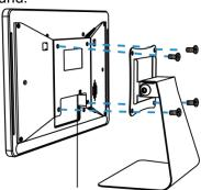
2. Fix the IoT Display to the VESA desktop stand by tightening the screws.
