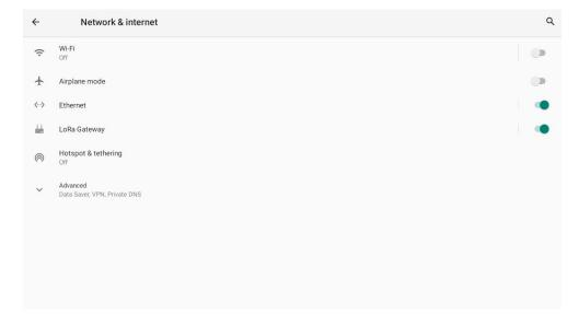
Select Ethernet IP mode as **static** or **dhcp** and plug the Ethernet cable to Ethernet port of device to access the network.
