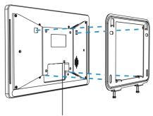
6. Fix the IoT Display to the bracket by tightening the 2 screws at the bottom of the bracket.
